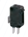
» Auxiliary contacts 1NO+1NC CODE D5LAU01 2NO+2NC CODE D5LAU02 Ie = 16 A (resistive loads) 4 A (inductive loads) at 250 Vac.
